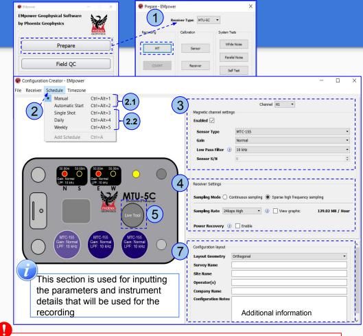
To use the magnetic sensor data from a different recording or use a remote reference, all recordings **must** have a matching Sampling Mode and Sampling Rates. Otherwise, EMpower will not allow to process data using borrowed channels or remote reference
